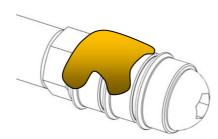
**STEP 5.** Withdraw the sampler body and slide & lock lid holder (3) to the end of the sampler shaft. Tighten onto shaft
