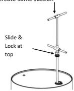
**ADJUSTMENT:** Suction strength can be adjusted by loosening the lock nut then turn bolt to apply more pressure to seals. Once completed re-tighten lock nut.
