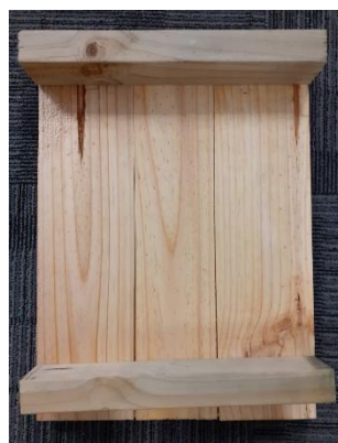
Bearers in position on top of base planks. 'Front' of the base is at the bottom of the photo.
