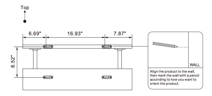
Note: The plastic inserts (#A1) are intended for concrete or cement block walls only. For drywall or hollow walls, substitute with a wood insert anchor (not included).
