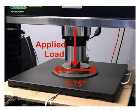
Figure 2: Test Setup 9.75" Distributed Load Test
