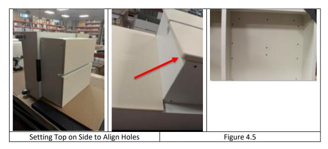
4.6. Set the sixteen (16) ¼-20 x ¾" button socket cap screws loosely in the holes beginning with the center two screws and working around to loosely set the rest using 5/32" hex head wrench. You may need to slightly adjust the positions of the Sub-base and Top as you go, taking care to set the screws straight and not
