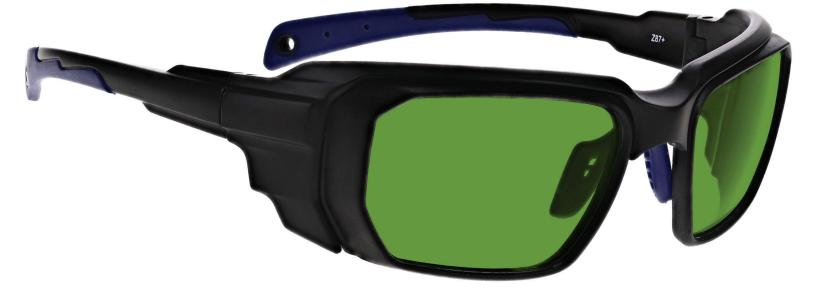
The Y97 laser safety glasses have a polycarbonate green lens filter that provides laser protection. These laser glasses have visible light transmission of 21%. In addition, the Y97 laser safety glasses have ANSI Z87+ plus ANSI Z136.1 safety standards. These laser safety glasses 16001 is a durable and lightweight wrap around frame. Made of high-quality plastic, the 16001 laser safety glasses feature adjustable nosepads. These Phillips Safety laser safety glasses are available in black/blue.
