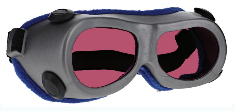
The AD laser safety glasses have a polycarbonate pink lens filter that provides laser protection. These laser glasses have visible light transmission of 32.6%. In addition, the AD laser safety glasses have ANSI Z87+ plus ANSI Z136.1 safety standards. These laser safety goggles 55 is a durable and lightweight fitover goggles frame. Made of high-quality plastic, the 55 laser safety goggles feature strap. These Phillips Safety laser safety goggles are available in silver.
