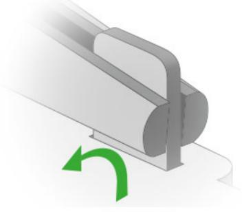
Use pliers to bend the fasteners
