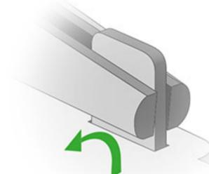
Use pliers to bend the fasteners
