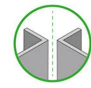
Assemble/bend parts symmetrically
