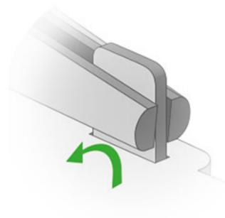
If there are no additional designa tions, Use pliers to bend the fasteners use the standard fixing method
