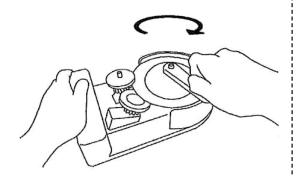
1) Do not apply excessive force to the crank while grinding.
