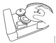
Align the pin on the back of the crank with the hole below.
