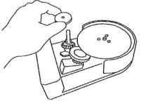
2. Make sure the hole on the circular blade is aligned to the hole on the crank. Insert the crank pins through the round blade and attach the crank.
