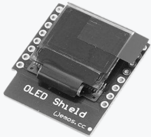
OLED Screen Optional module which can be installed atop the Wemos D1 MCU
