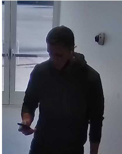
Poor lighting (50 lux on subject)
