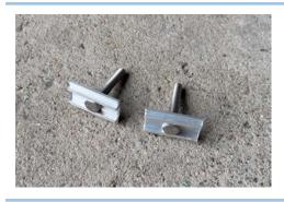
10. Setup the sandwich plates by placing a bolt in each plate
