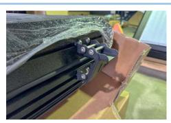
7. Clip the latch hooks onto their mounting point, Once ALL the canvas is tucked under the rubber seal
