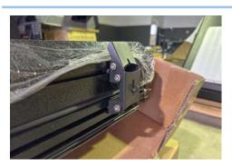
8. Press upwards on the latches to fully close the tent.
