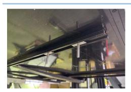
12. Slide in the two sandwich plates with bolts into the chanel, centre above crossbar of roof rack
