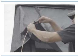
7. Hook the other end of the pole into the awning eyelet
