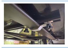
14. Fit remaining 'U' plates and nuts to clamp the tent to the roof rack
