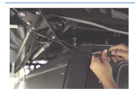
12. **OPTIONAL:** Plug in the supplied lighting connector to a 12v source
