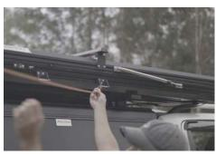
6. Hook the other end of the tensioner rope onto your roof rack, tent etc. Leave loose
