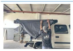
8. Push the frame flush with the backboard of the awning bag
