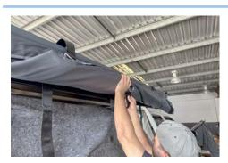
12. Whilst holding the rolled up canvas, bring the velcro strap through the loop and tightly stick it back to itself
