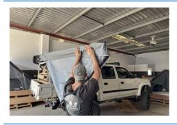
5. Pulling the rope, walk the awning around the car
