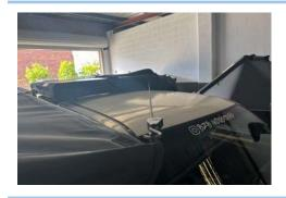
9. Hook the other end of the tensioner rope onto your roof rack, tent etc
