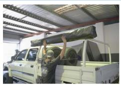
6. Lift the awning up to the car, lining up the bolts to the awning brackets
