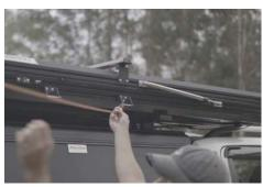
6. Hook the other end of the tensioner rope onto your roof rack, tent etc
