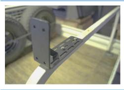
4. Bolt the supplied awning bracket to your roof rack / roof cage
