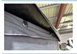
10. Where the loops are for the velcro, reach behind the awning frame and feel for the velcro strap
