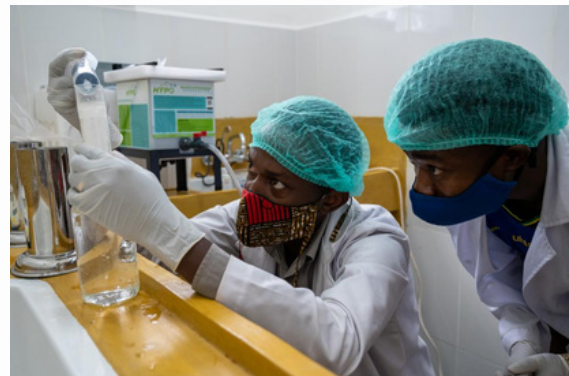
Staff at FAME Hospital are trained in how to prepare hypochlorous acid in the Hypo 7.5.
