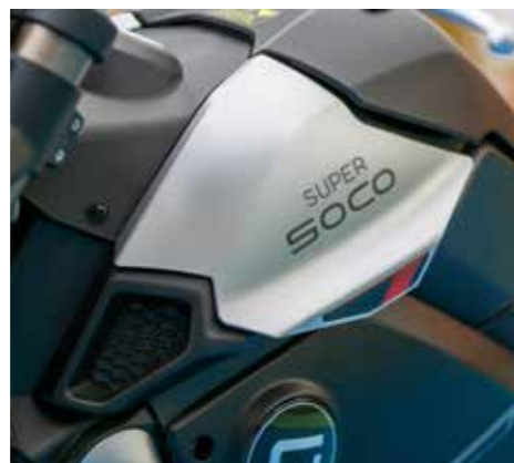
In de zogenaamde 'tank' vinden we de dikke 72V/45Ah accu
