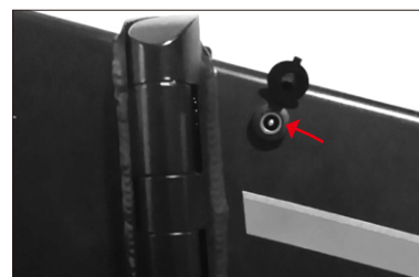
Battery charging port
