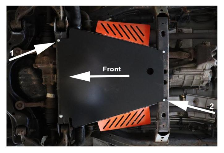
**Step 5:** Using a floor jack, lift the new transmission skid plate into position as shown above. The wide part of the skid plate fits toward the front of the truck and between the chassis and the oil pan skid plate, if equipped.
