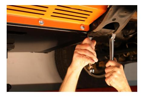
**Step 6:** With the 3/8-16 UNC hex head bolt tightened, the nut plate's location is now determined. Tighten the crossmember bolt holding the nut plate. A wrench can be slipped between the skid plate and the crossmember to hold the nut. Use a ratchet wrench on the head of the bolt as shown in the photo above.
