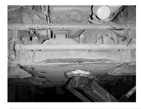
**Step 2:** Position the engine/transmission skid plate under the vehicle so that the leading edge of the skid plate is facing forward. The leading edge has three nuts welded in place to its top surface. Place the skid plate on a floor jack and raise it so that the leading edge of the skid plate extends a little forward of the crossmember that supports the front differential.
