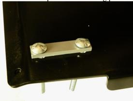
**Step 4:** Insert the carriage bolts through the slotted holes in the front of the skid plate and to the front and back of the crossmember. Place a round hole retaining plate over the carriage bolts across the top of cross-member and install the 3/8-16 nuts and lock washers finger tight. Then install the other set.
