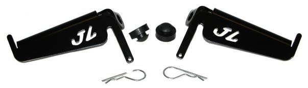
**Step 1:** Using a little liquid soap, push the rubber bumper into the hole on each foot peg. It's helpful to twist the bumper a little to get it into the hole.
