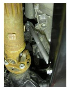
**Step 10:** Install the driver's side strut rod as shown at left, again using one of the 3/8-16 x 1.5" bolts at the top of the strut rod and one 3/8-16 x 1" bolts at the bottom. Make sure to place the strut rod within the skid plate as shown. Also, please note that the strut rod isn't quite symmetrical. It will fit better one way than it does the other, but there is no distinguishing feature for top or bottom.
