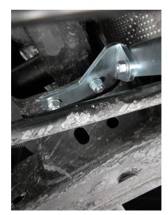
**Step 3:** Install the passenger side-mounting bracket using the bolts just inserted into the motor mount. The mounting tab faces the rear of the vehicle. It is shown with the strut rod attached in the photo to the left. Leave these bolts loose for now.
