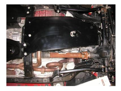
**Step 7:** Using a floor jack (or a friend) position the skid plate as shown above.
