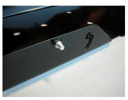
**Step 3:** Place three of the carriage bolts through the holes on the side of the skid plate with the Skid Row logo cut out as shown in the photo at left. Their threads should face outward. Put a nut on each one to keep it in place while positioning the skid plate.
