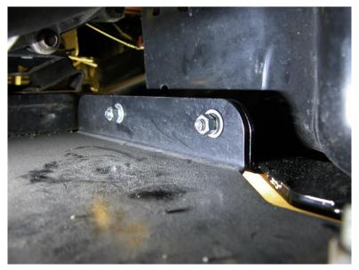
**Step 9:** Re-install the factory mounting bolt for the transfer case skid plate through the gas tank skid plate. The ½" thick aluminum spacer is used between the gas tank skid and the mounting bracket of the transfer case skid plate.
