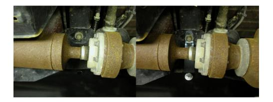
**Step 7:** The Mounting Bracket w/o Nut is installed at the rear, outboard side of the skid plate, near the Skid Row logo. Again, remove the factory skid plate mounting bolt from the chassis. Then remove the nut that was installed on the carriage bolt. Place the bracket over the carriage bolt and install the flat washer, lock washer, and nut. Then re-install the factory mounting bolt through the bracket as shown.
