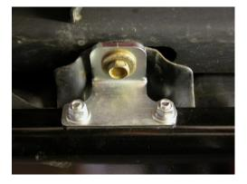
**Step 6:** The 7" Mounting Bracket with Nut is installed at the rear, inboard side of the skid plate. Remove the factory mounting bolt that is above the slotted hole. Place the bracket in position and install one of the 3/8-16 x 1" Hex Head Bolts, a flat washer, and a lock washer through the skid plate into the nut on the bracket. Then re-install the factory mounting bolt.
