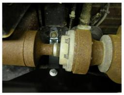
**Step 8:** The Mounting Bracket w/o Nut is installed at the rear, outboard side of the skid plate, near the Skid Row logo. Again, remove the factory skid plate mounting bolt from the chassis. Then remove the nut that was installed on the carriage bolt. Place the bracket over the carriage bolt and install the flat washer, lock washer, and nut. Then re-install the factory mounting bolt through the bracket as shown.
