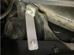
**Step 9:** Use the remaining two carriage head bolts, flat washers, lock washers, and nuts to attach the gas tank skid plate to your Skid Row Offroad transfer case skid plate as shown below.
