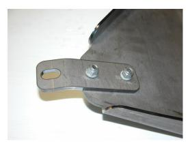
**Step 2:** Install the bent mounting bracket to the driver's side of the skid plate using two of the 1" carriage bolts as shown at left. Leave the bolts loose.
