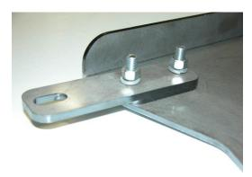
**Step 3:** Install the flat mounting bracket to the passenger side of the skid plate using the two 1.5" carriage bolts. Place the 3/16" thick, 2 hole spacer between the skid plate and the bracket as shown at left. Leave the bolts loose.
