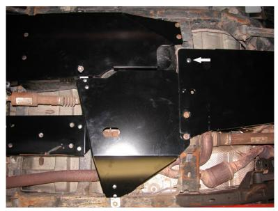
**Step 8:** If using our gas tank skid plate, install the two 3/8-16 nuts, flat washers, and lock washers to the two carriage bolts that hold the transfer case skid plate to the gas tank skid.
