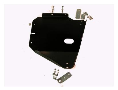
**Step 1:** Remove the factory Transfer Case skid plate and retain the four bolts. They will be re-used.
