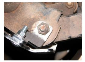
**Step 6:** Put one of the nut plates inside the shock mount with the nuts facing upward.
