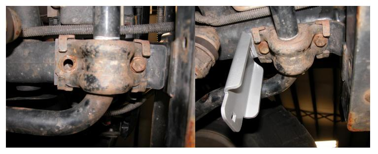
**Step 3:** Install the two mounting brackets by slipping them into place between the sway bar mounts and the chassis. Reinstall the two bolts removed in Step 2 and then tighten all four bolts.
