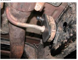
**Step 16:** Place the Exhaust Hanger Adjuster over the exhaust hanger pins as shown in the photo to the left. This "locks" the two pins together to facilitate bending the frame mounted pin upward in the next step.
