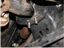
**Step 3:** Install the passenger side-mounting bracket using the bolts just inserted into the motor mount. The mounting tab faces the rear of the vehicle. It is shown with the strut rod attached in the photo to the left. Leave these bolts loose for now.
