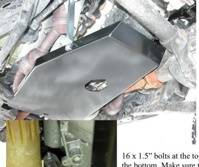
**Step 7:** Using a floor jack (or a friend) position the skid plate as shown at left.
