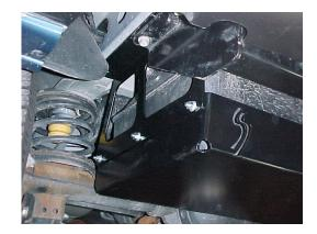
**Step 4:** If your Jeep has a hitch slide it into place as shown in the photographs above and install using the hardware supplied with the hitch. Be sure to place the 3/16" thick spacer between the hitch and the "frame rail" on the passenger side if your hitch uses the forward-most bolt hole. Torque the bolts to the hitch manufacturer's recommended torque.
