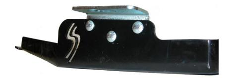
**Step 2:** If your Jeep has a front skid plate, loosen the four mounting bolts. On 2002-2004 models, also remove the rearmost bolt that is on the angled surface. If your Jeep **does not** have the factory front skid plate, install two of the M10-1.50 bolts with washers in the threaded holes in the frame as shown below. You may find it necessary to run a tap through the threaded holes in order to clean rust and debris out of the threads.
