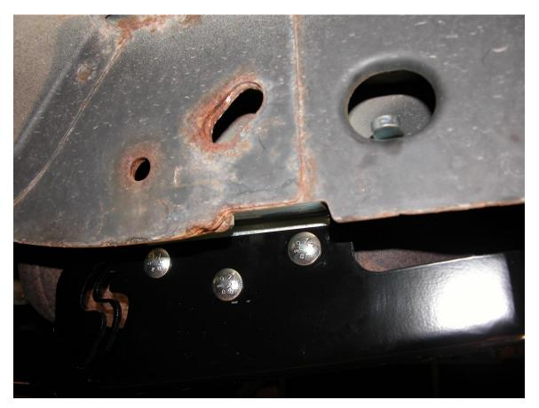
**Step 7:** Bolt the bracket to the "chassis" using the remaining M10-1.50x35mm bolt, lock washer, and flat washer.
