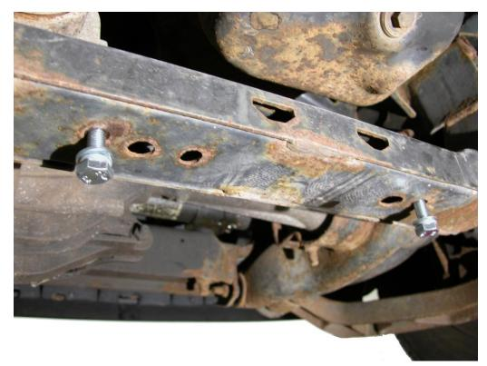
**Step 3:** If your Jeep has a factory transfer case skid plate both of the bolts that hold it to the transmission cross-member will need to be removed. Skip to Step 4.
