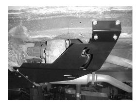
**Step 1:** Place the skid plate up against the frame rail and the transmission cross-member in the position shown. The three square holes in the skid plate should line up with holes in the cross-member for most XJ's.
