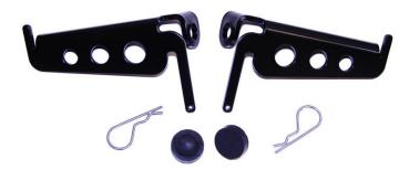
**Step 1:** Using a little liquid soap, push the rubber bumper into the hole on each foot peg. It's helpful to twist the bumper a little to get it into the hole.
