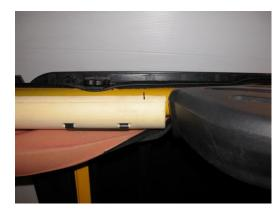
**Step 2:** Mark the location on the bar and on the padding where you want to place the Top Prop. It should be roughly centered above the door. On vehicles with a sound bar, place the socket just behind the sound bar as shown in the photo. Then remove the foam padding from the tube being careful not to break the foam. There are plastic fasteners along the bottom of the padding that you simply pull out of holes in the roll bar tubing.
