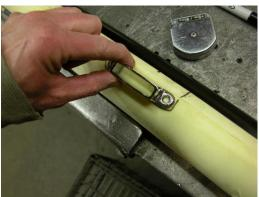
**Step 3:** Place a bow socket along the top edge of the padding, centered on your mark, and draw a line around it as shown above left. Then place the socket along the line you just drew and draw a second line around the socket as shown in the photo above right. Then cut away the padding material along the lines just made.
