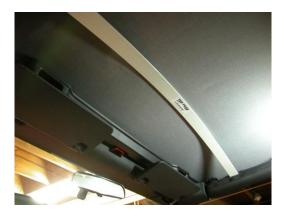
**Installing the Slat:** Simply insert one end of the slat into one of the bow sockets, push the slat up in the middle, and insert the other end of the slat into the other bow socket. That's all there is to it!
