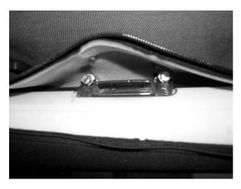
**Installing the Screws:** The clamps can be removed and replaced by the sheet metal screws provided, if desired. However, it is not necessary to perform this step since the clamps will hold the Top Prop in place permanently. They will also allow you to remove your Top Prop easily using only a straight-blade screwdriver.
