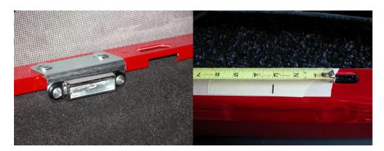
**Step 3:** You will need to mark and drill four holes to install the mounting brackets. Measure 3" from the hole on top of the tub roughly in the middle of the soft top window. The dimension isn't critical, but it is important to make sure that you avoid the wiring harness, mounting tabs, and carpet. The carpet fits snugly on the sides, but can be pulled out of the way. It's also a good idea to use the same dimension from one side to the other.
