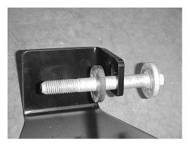
**Step 3:** Start with the driver's side skid plate. On all models except 2003-2006 TJ and LJ's simply put the <sup>1</sup>/<sub>4</sub>" thick washer in your can of spare nuts and bolts. It isn't needed. On 2003-2006 model TJ and LJ's slide the control arm bolt you removed in Step 2, through the skid plate and then place the washer over the bolt as shown in the picture to the left.
