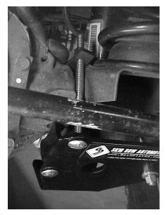
**Step 9:** For vehicles equipped with cam bolts turn the bolt head until the marks you made earlier line up. Holding the head from turning, torque the nut on the lower control arm mounting bolt to the recommended torque. Sorry, but we can't give a number for this since it varies based on model year and whether or not you are using factory or after-market control arms.
