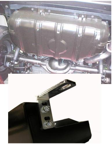
**Step 2:** Insert the remaining two 5/16-18x1.0" carriage bolts into the two square holes at the front of the skid
