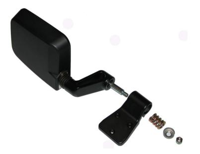
**Step 4:** Mount the mirror into the new mirror relocation bracket using the cup washer or the 1.25 fender washer and the original nut. Position the mirror and tighten the nut.
