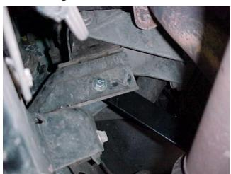
**Step 7:** Take the strut rod and attach it between the motor mount and the skid plate. Use one 3/8-16 bolt, lock washer, and nut to bolt it to the front of the skid plate and use the remaining ½-13 bolt, washer and nut to attach it to the rear of the motor mount. The view in the photo to the left is from the rear on the driver's side.
