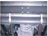
**Step 5:** Lift the engine skid plate and slide it over the threaded portion of the lower control arm bolt. Position the rear edge of the engine skid plate within the notched out area on the factory transfer case skid plate as indicated by the arrows in the picture to the left.
