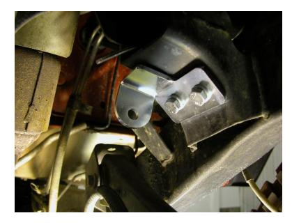
**Step 4:** Take the mounting bracket and attach it to the bottom of the motor mount using two of the 3/8-16 bolts with lock washers with the tab to the rear of the vehicle. The view in the picture above is looking from the front. **NOTE: The tab MUST be to the rear of the vehicle or control arm damage could result.**
