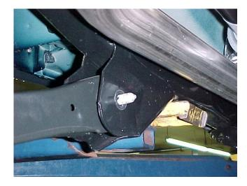
**Step 3:** Take the T-shaped nut plate and slide it into the driver's side motor mount through the top opening. Once the nuts can be seen through the two holes in the lower side of the motor mount, the tab may be folded over to hold the nuts in position. It is helpful to give the tab a slight arch before inserting it into the motor mount.
