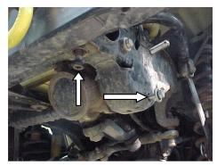
**Step 1:** Remove the two bolts indicated in the picture to the left.
