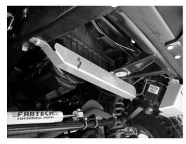
**Step 3:** Align the radiator guard with the lower tank of the radiator. Mark and then drill a 5/16" hole into the passenger side of the frame using the hole in the guard as a guide.
