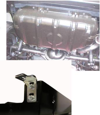
**Step 2:** Loosely attach both rear mounting brackets to the skid plate using the 5/16-18x1.0" carriage bolts, 5/16-18 nuts, and washers provided. The bolts should be installed from the inside of the skid plate. The longer bracket is installed on the passenger side of the vehicle to reach over the exhaust pipe.
