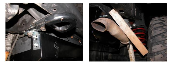
**Step 9:** You may find that you need additional exhaust system clearance as shown in the photo below left. Simply bend the exhaust hanger bracket shown below right to gain this clearance. You can also remove the threads that are protruding past the nut with a hacksaw.
