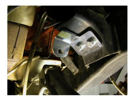
**Step 3:** Take the mounting bracket and attach it to the bottom of the motor mount using two of the 3/8-16 bolts with lock washers with the tab to the rear of the vehicle. The view in the picture above is looking from the front. **NOTE: The tab MUST be to the rear of the vehicle or control arm damage could result.**
