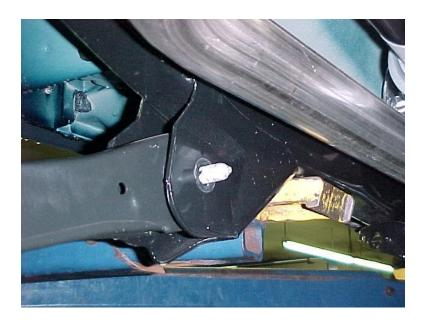
**Step 2:** Take the T-shaped nut plate and slide it into the driver's side motor mount through the top opening. Once the nuts can be seen through the two holes in the lower side of the motor mount, the tab may be folded over to hold the nuts in position. It is helpful to give the tab a slight arch before inserting it into the motor mount.
