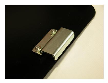
**Step 4:** Take the engine skid plate and loosely attach the transfer case skid plate clamp using two 3/8-16 bolts with lock washers. Be sure that the hook shaped portion of the clamp is facing the back of the skid plate as shown above.
