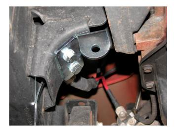
**Step 3:** Repeat steps 1 and 2 on the passenger side motor mount. On the passenger side, the T-shaped nut plate is more easily inserted from the bottom of the motor mount as shown above. The view above is from the front. **NOTE:** On the passenger side the tab MUST be towards the front of the vehicle.
