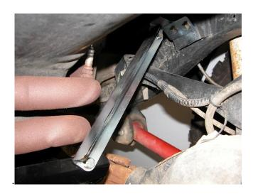
**Step 4:** Take the driver side strut rod and attach it between the mounting bracket and the skid plate on the driver side. **NOTE: The driver side strut rod is the longer of the two.** The end of the strut rod with the tab should be near the motor mount. Use one 3/8-16 bolt, lock washer, and nut to bolt it to the front of the skid plate and use another bolt, lock washer, and nut to attach it to the mounting bracket on the motor mount. Attach hardware loosely and do not tighten at this time
