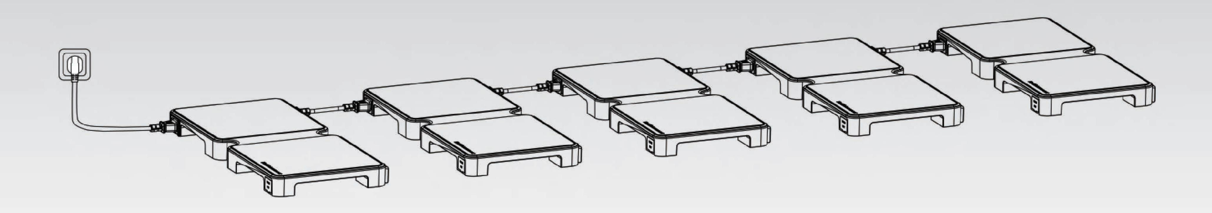
Your **HotMat Connect** can connect up to 5 identical units using only one socket connection. To connect an additional unit, use the dedicated connecting cable and attach it first to the 3-pin insert of the additional unit to be added. Then connect it to the opposite insert of the original unit. To connect more units (up to 5 units only), repeat this process and connect each additional unit it to the preceding unit.
