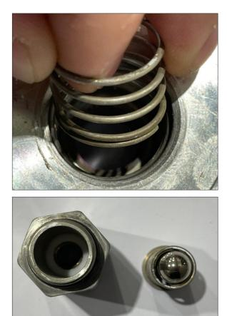
**Step 11:** Remove the spring over the upper loader-seal.
