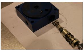
**Step 5:** Use a pick to push the sleeve out of the upper air drive cap.
